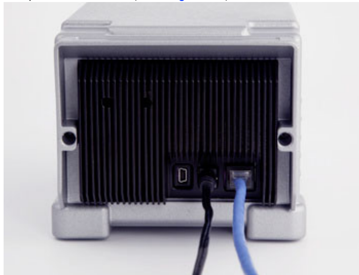
Figure 2-5 FlowIR—Power and communications connected
