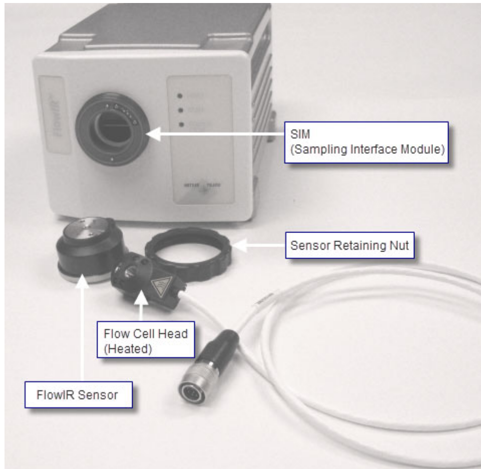
Figure 2-6 FlowIR with heated flow cell sampling technology
