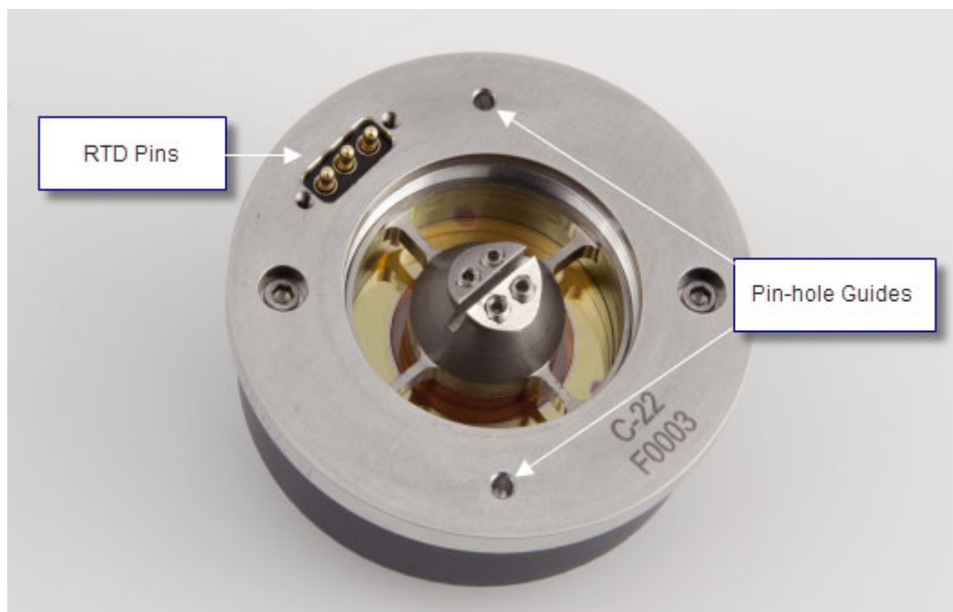
Figure 2-7 FlowIR Sensor—RTD connection pins (3) and pin-hole guides (2) to base unit
